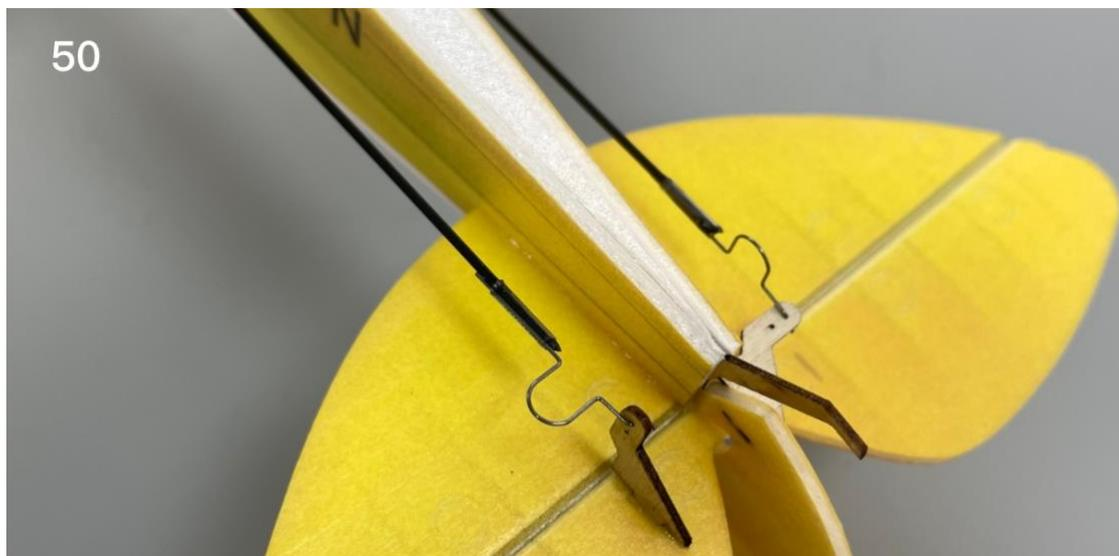
51. Attach the steel wire hooks to the aileron control horns.
