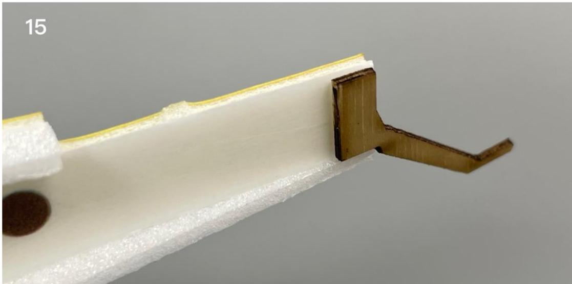
16. Bend the nose cover parts along the scribed line on the inner side.
