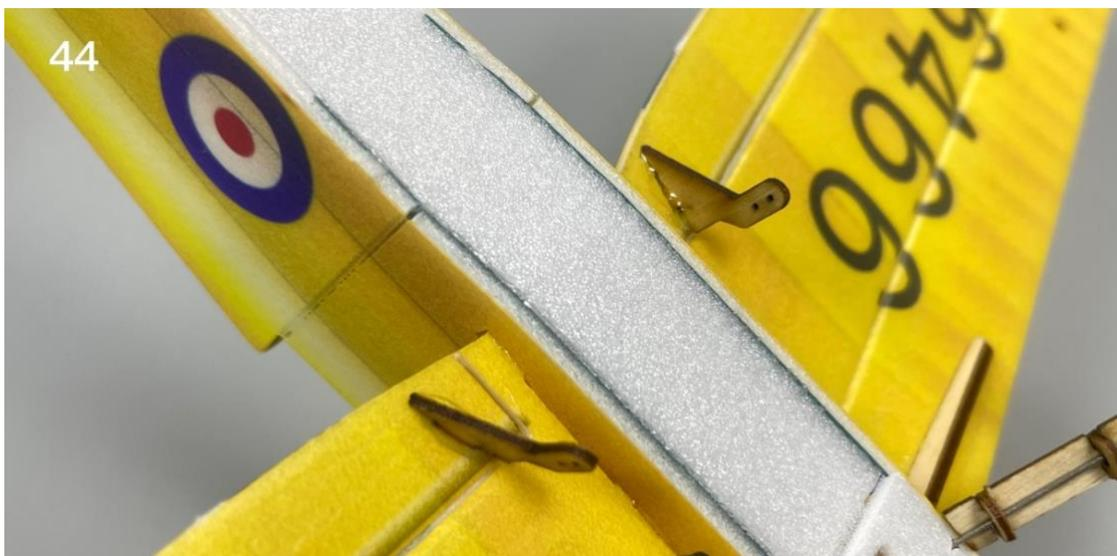
45. Install rudder and elevator control horns.
