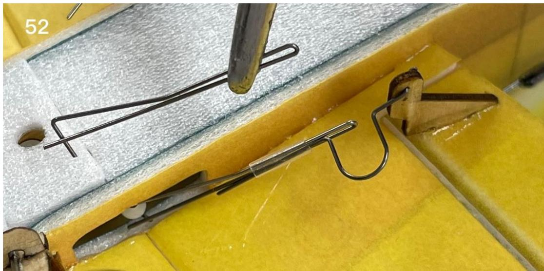
53. Connect the aileron steel wire hooks and clips with heat shrinkable tubes on both sides.
