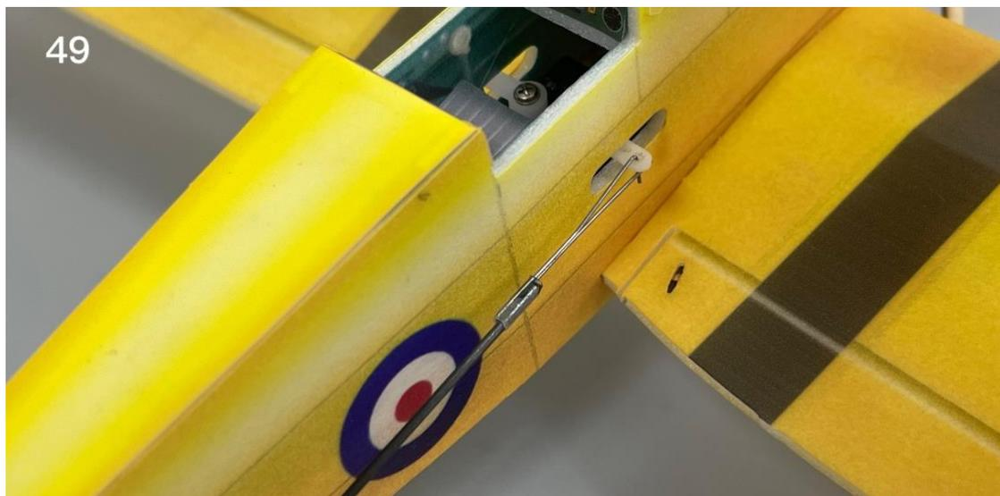
50. Cut the carbon rod to proper length and connect the wire hooks with heat shrinkable tubes.
