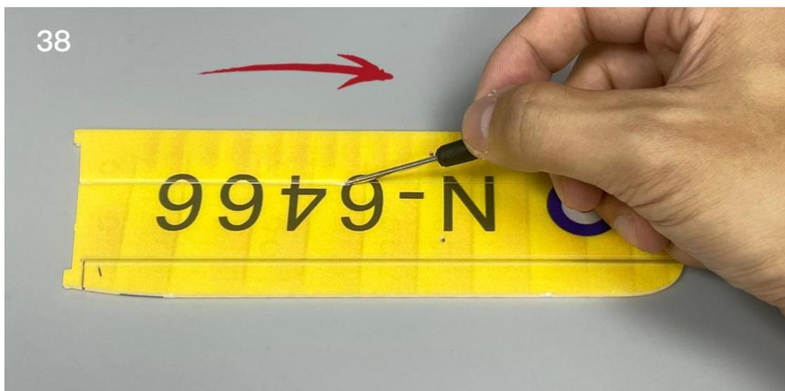
39. Use the end of a screw driver to score through the aileron half-cut line of the aileron.
