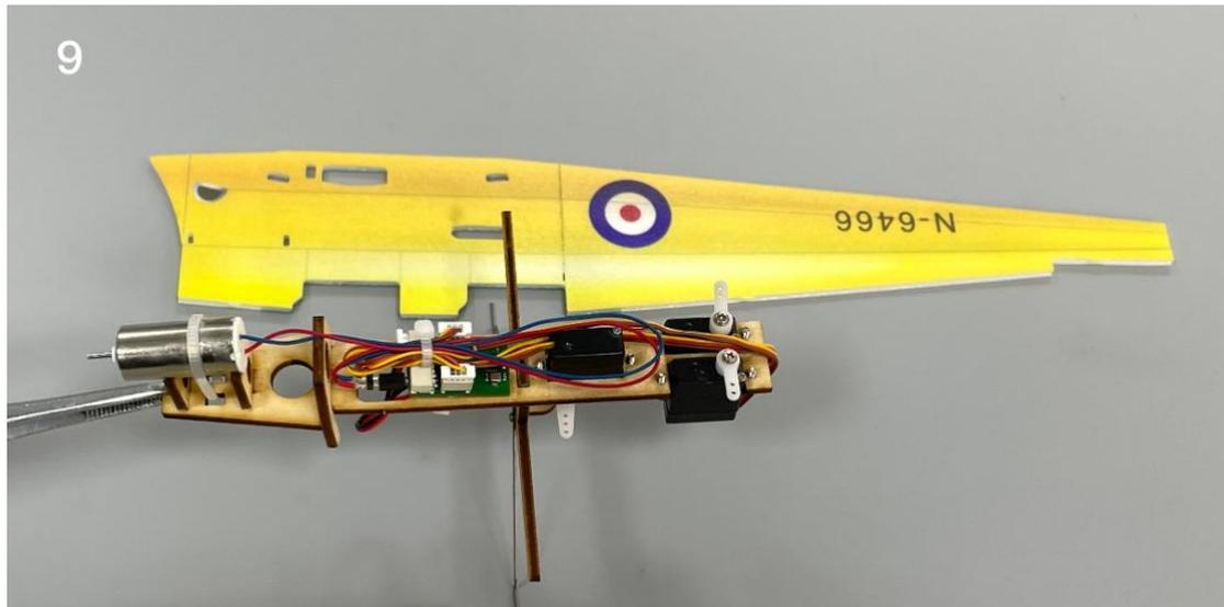
10. Align the scribed line on the inner side of the fuselage and fix the wooden structure with glue.
