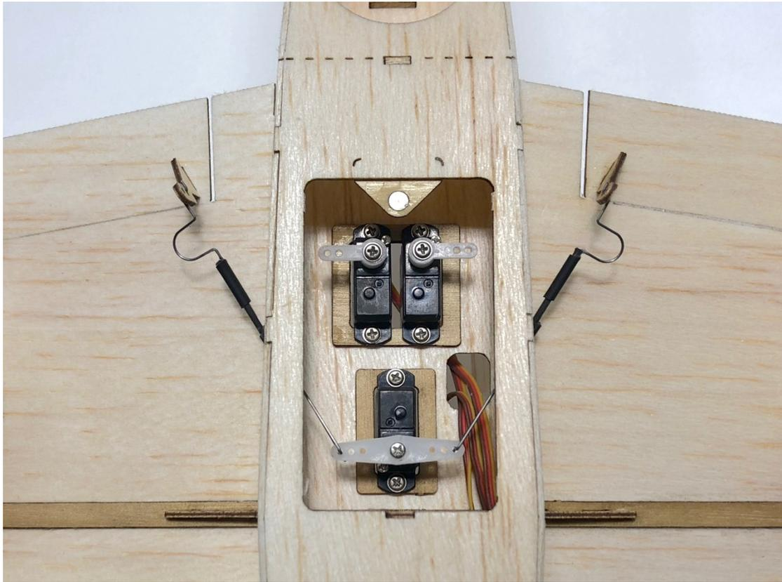
56. Connect the pushrod clips & pushrods with heat shrinkable tube and fix them with glue.
