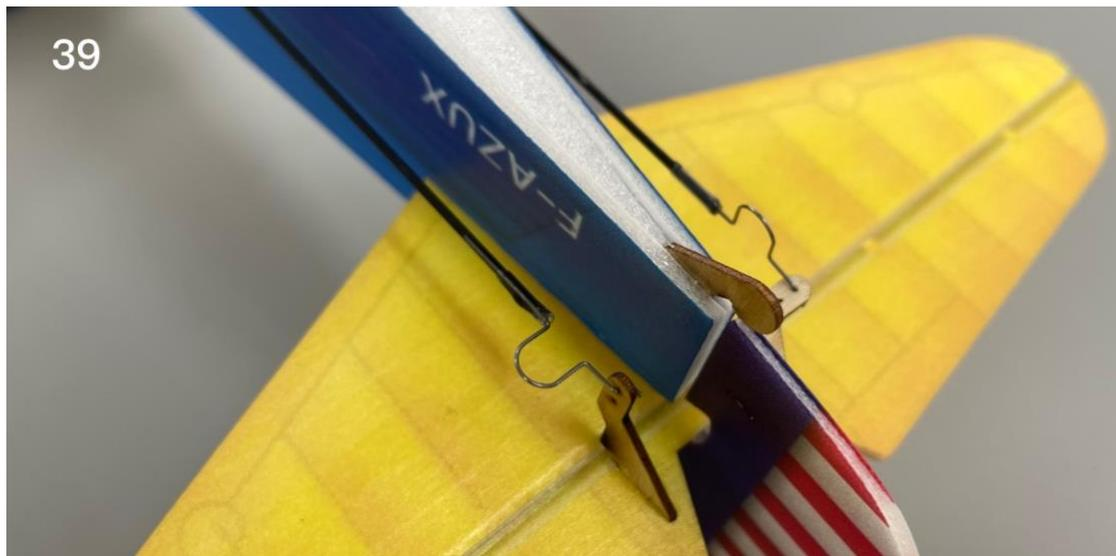
40. Attach the steel wire clips to the aileron servo arms.
