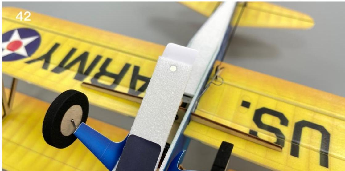
43. Fix the battery cover magnet with glue and cover it with stickers.
