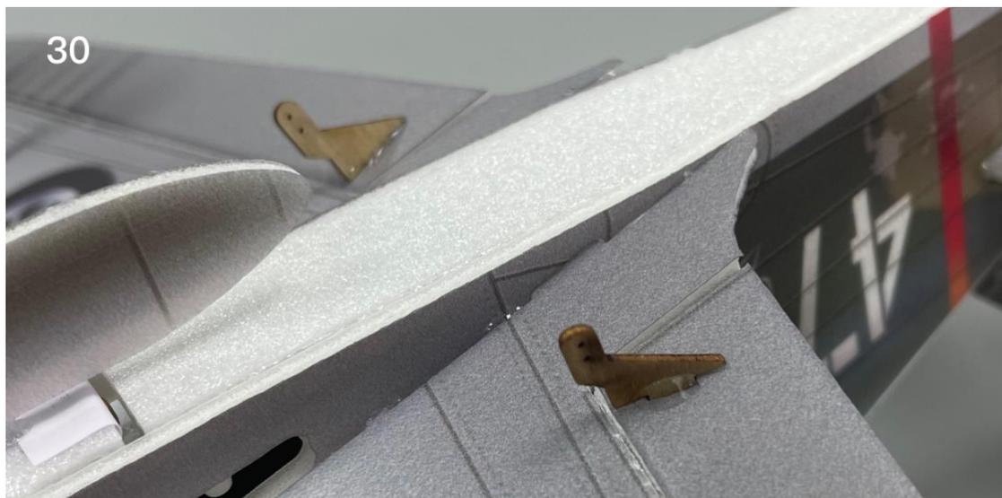
31. Install rudder control horns.
