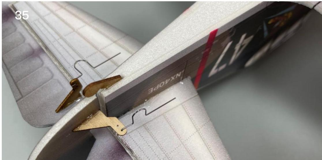
36. Cut the carbon rod to proper length and connect the wire hooks with heat shrinkable tubes.
