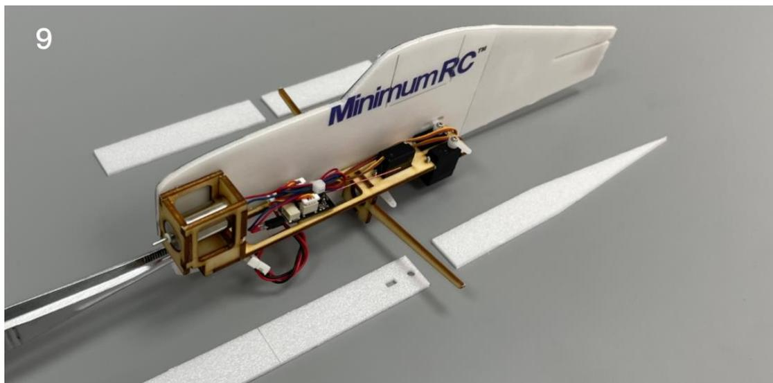
10. Note: the position shown in the picture is the battery cover plate that can be opened. No glue shall be applied to the area marked by the yellow line.
