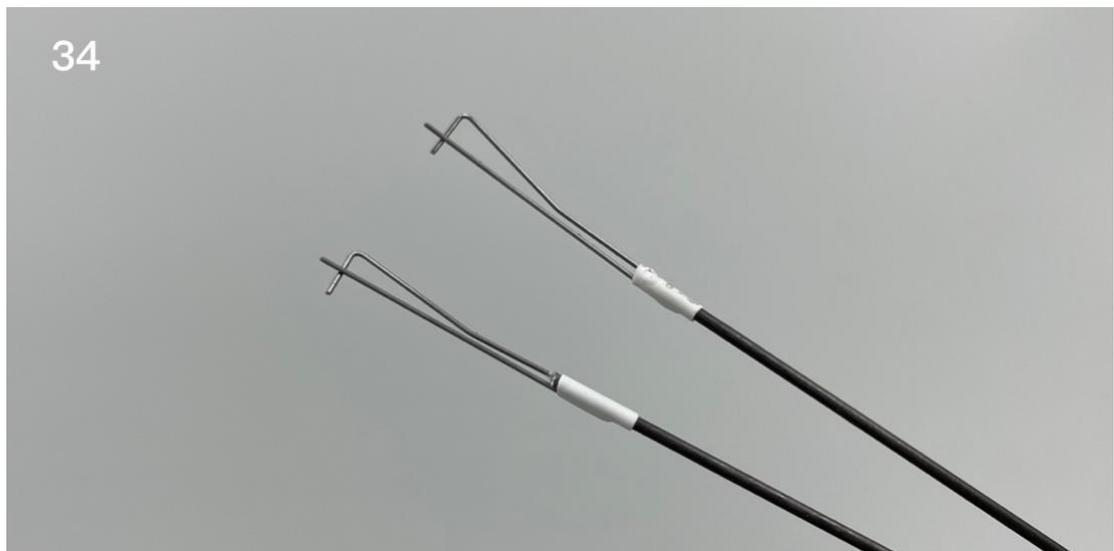
35. Attach the steel wire hooks to the control horns.
