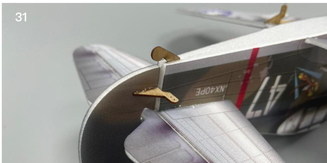
32. Install elevator control horns.
