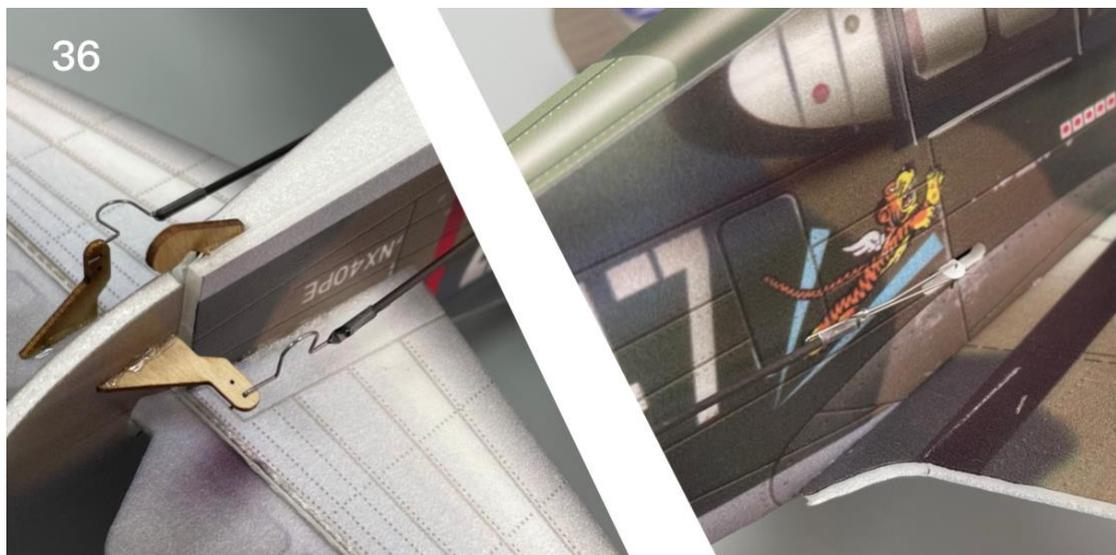
37. Use heat shrinkable tube to connect aileron steel wire clips & hooks.
