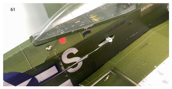
62. Trim the carbon fiber rod to the appropriate length. Use heat shrink tubing to connect the carbon fiber rod to the connection hook, then apply 502 glue for
