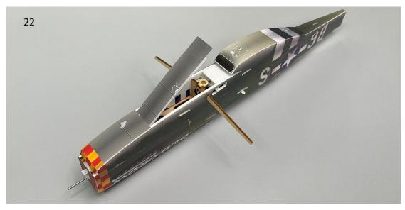
23. Install magnets at the circular hole position of the battery compartment cover.
