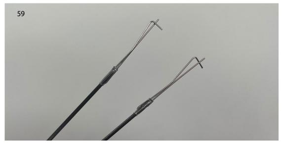
60. Install connection hooks on the tail control horns.
