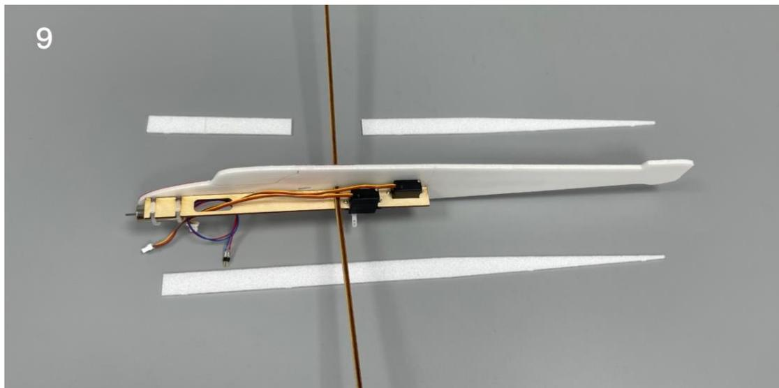
10. Fix the top and bottom strip of the fuselage with glue.
