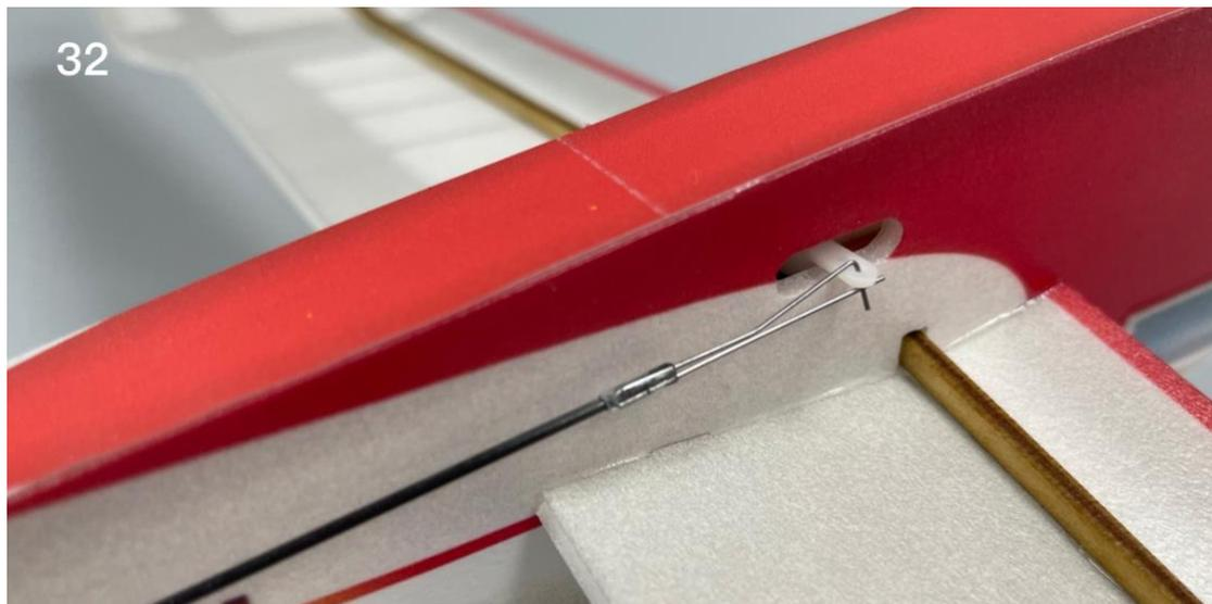
33. Connect the steel wire hook and the push rods with heat-shrinkable tube.
