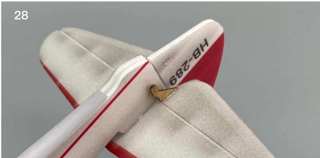
29. Attach the steel wire hook to the control horns.
