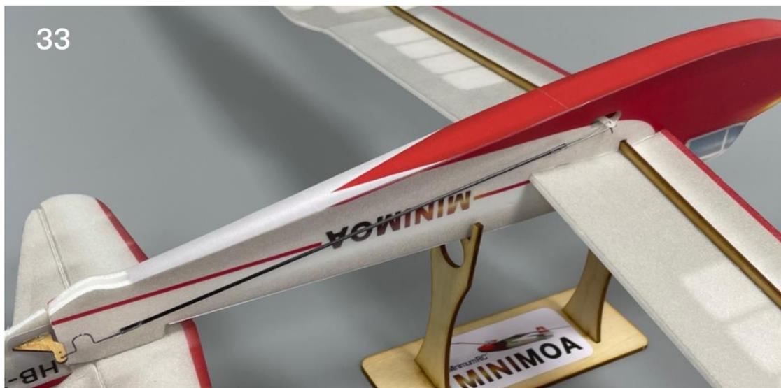
34. Connect the steel wire hook and the push rods with heat-shrinkable tube.
