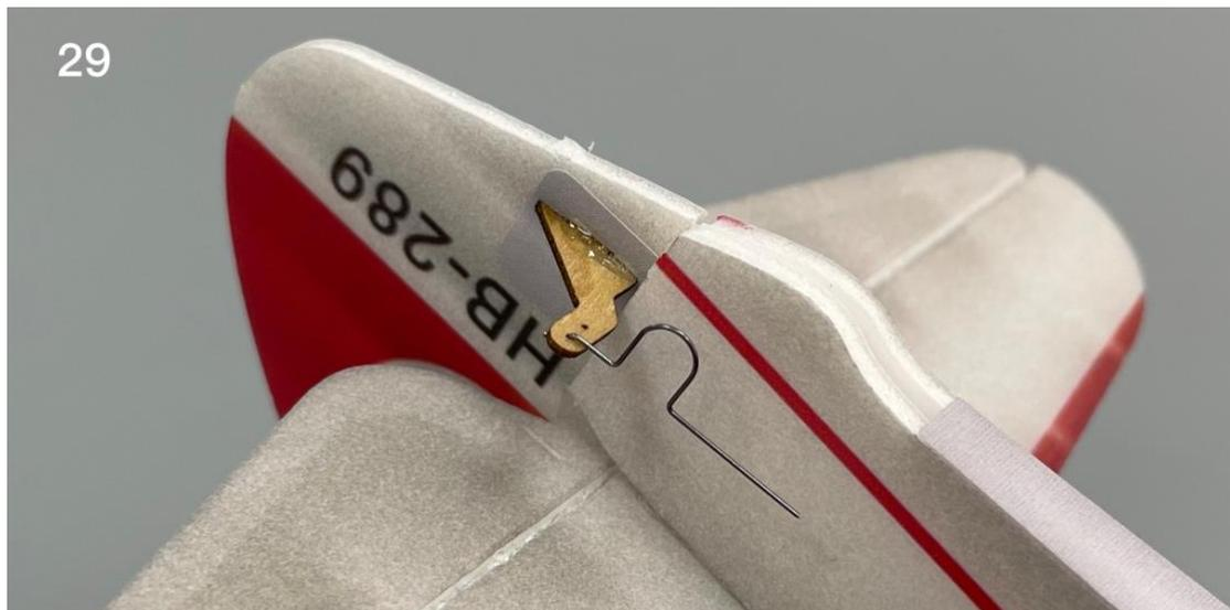
30. Attach the steel wire hook to the control horns.
