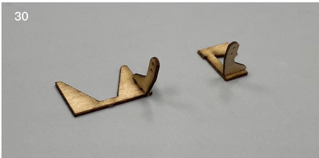
31. Glue the control horn parts on the tail. Please make sure that the elevator and rudder can move freely.
