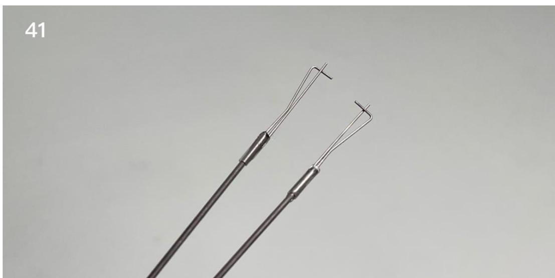
42. Extend the carbon rod of the pull rod from the slot at the middle and rear of the hull, and use tweezers to fasten the steel wire clamp on the hole of the servo arm.
