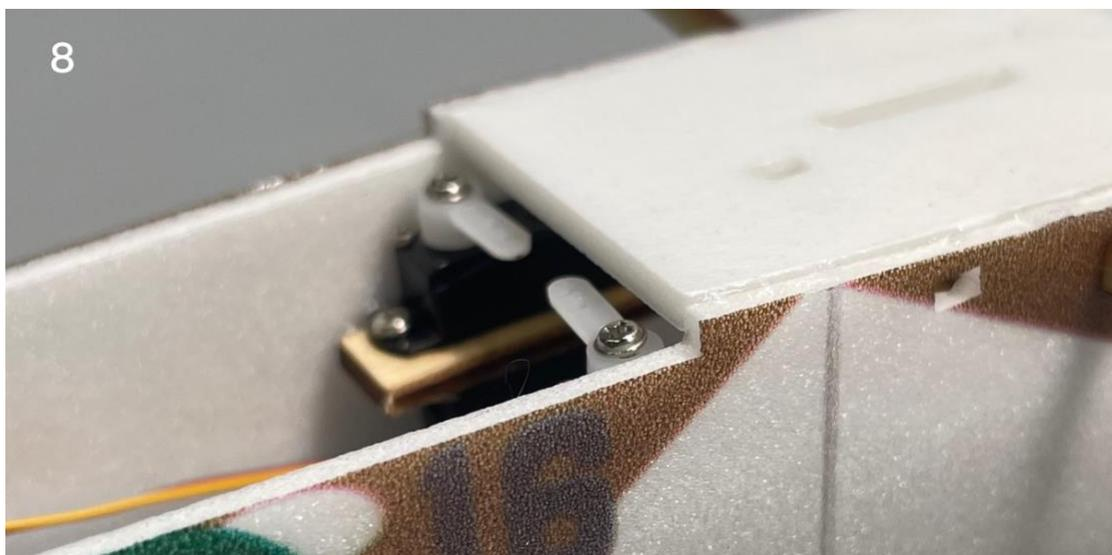
9. Details: there should be a gap between the middle part of the hull and the tail roof to allow the push rod to pass through.
