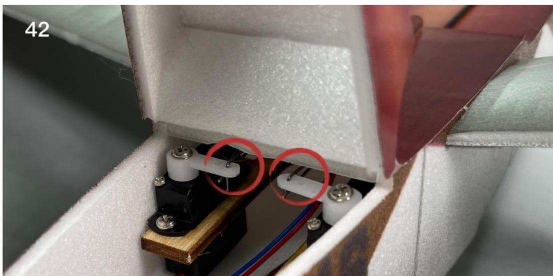
43. Details: the carbon rod of the pull rod extends from the slot in the middle and rear of the hull.
