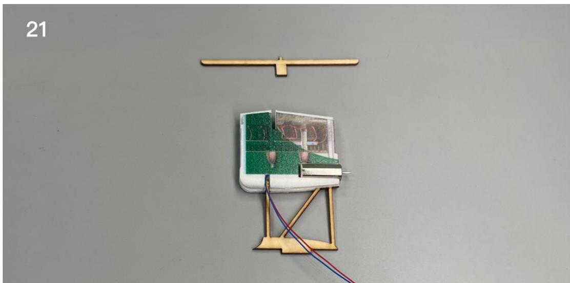
22. Install the spar. Please keep the spar perpendicular to the motor base.
