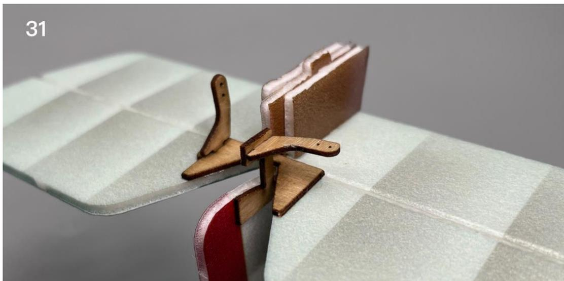
32. Install the tail assembly and paste the tail side sticker. Make sure the horizontal tail is parallel to the fuselage and the vertical tail is vertical to the fuselage
