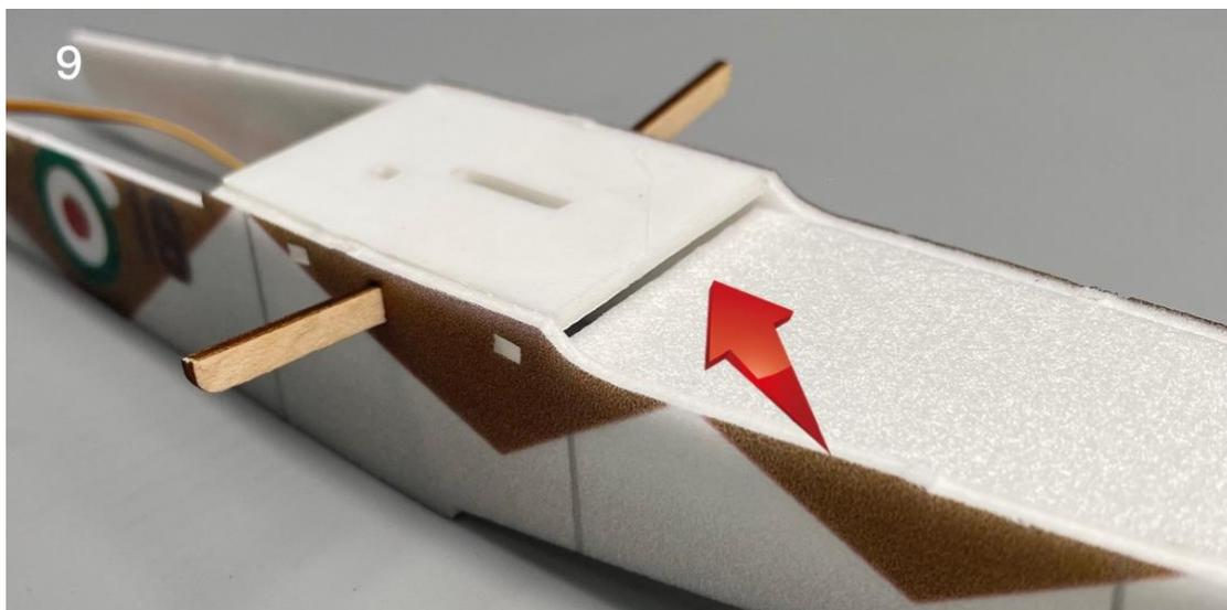
10. To install the bottom plate of the hull head, the plate can be bent in advance before installation.
