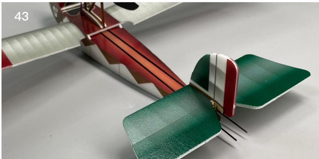
44. Install the rudder angle wire clamp on the control horn hole. Cut off the excess length of the carbon rod, connect the steel wire with the carbon rod with a heat shrinkable tube, and drip 52 glue to fix it.
