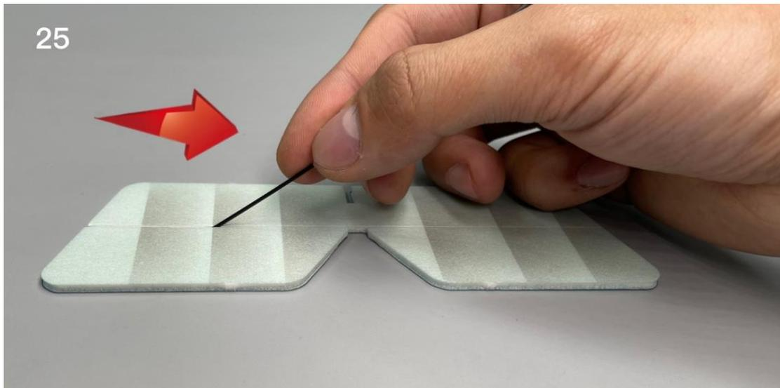
26. Use the end of a carbon fiber rod to score through the half-cut line of the rudder surface.
