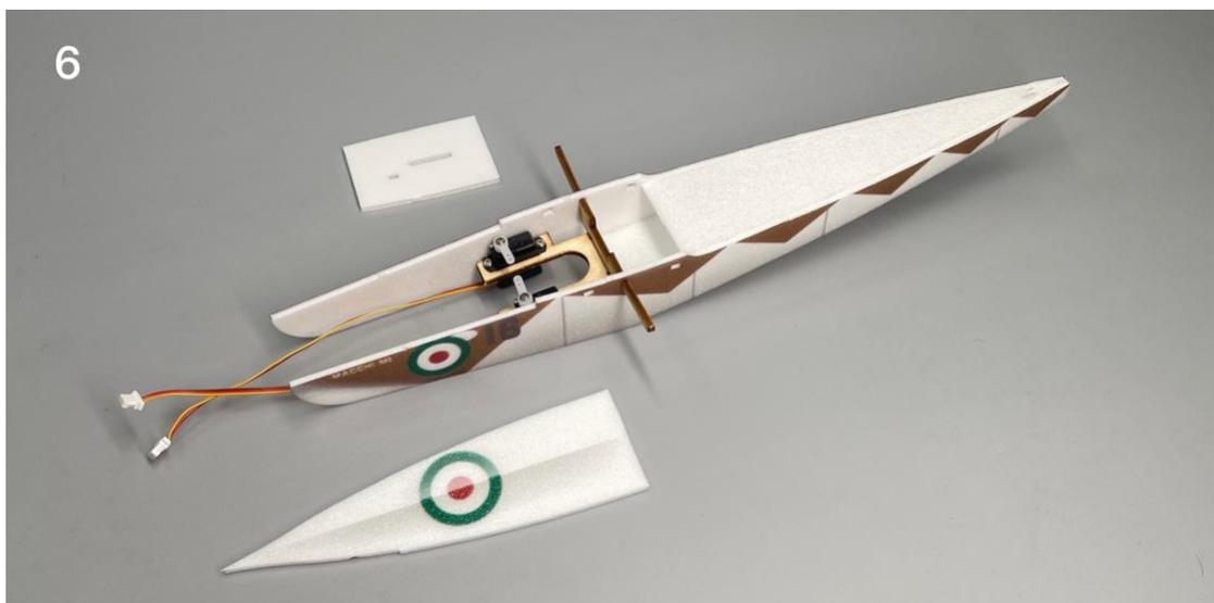
7. Install the top plate of the middle part of the hull with a small hole and one end facing forward.
