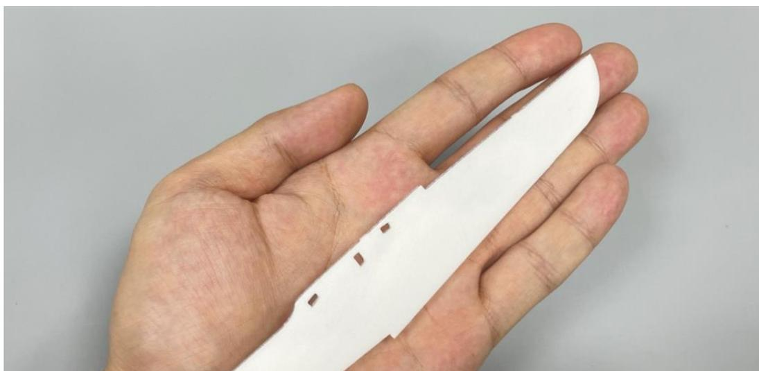
Press the position where the part needs to be bent on the edge corner of the desktop, keep the palm close to the part, and slide down.
