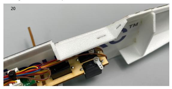
21. Use glue to secure the nose filler plate.
