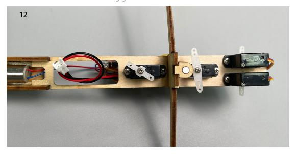
13. Connect the receiver to the servos, secure the receiver with Velcro, power it on, and bind it to the transmitter to ensure that the servo arms return to their neutral positions. Test if the servos are functioning correctly and install the servos and arms as shown in the diagram. Note: This step is crucial; make sure the servos are powered, the arms are centered, and follow the diagram precisely. Adjustments cannot be made after the model is assembled.
