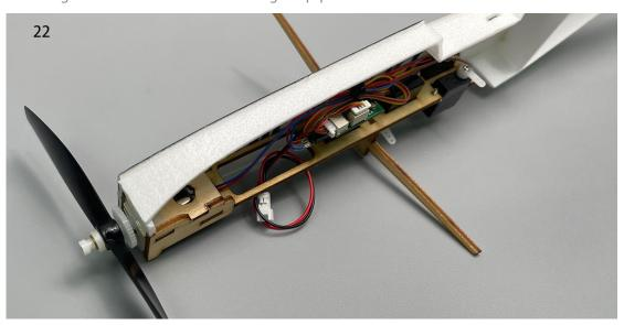
23. Use glue to secure the fuselage bottom plate, do not apply glue to the red-lined section.
