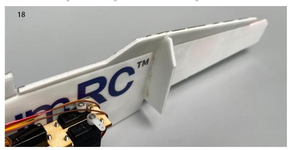
19. Use glue to secure the foam board at the bottom of the tail of the aircraft.
