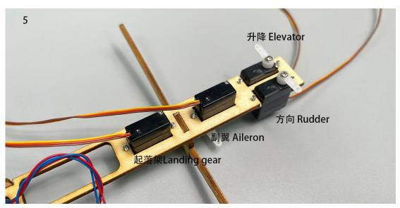
6. Install the servo as shown. (Bottom view of the parts)
