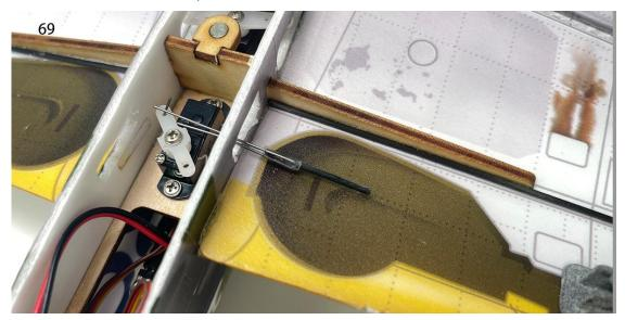
70. Install the landing gear drive rod into the groove.
