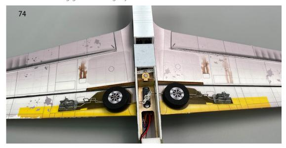
75. Adjust the landing gear wires so that they are vertical to the ground when in the open position.
