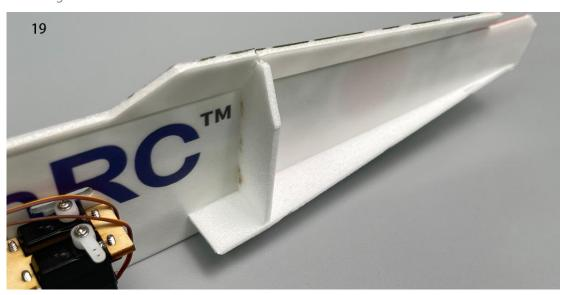
20. Use glue to secure the cockpit foam board.
