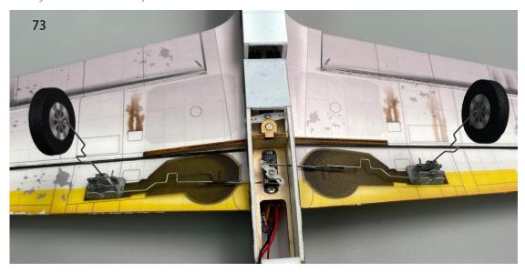
74. Bend the landing gear wires slightly towards the front of the aircraft.
