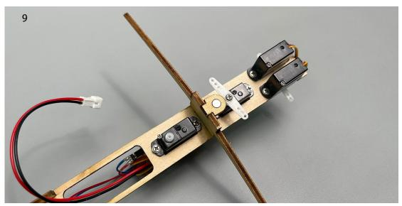
10. The landing gear servo uses a cross-shaped arm.
