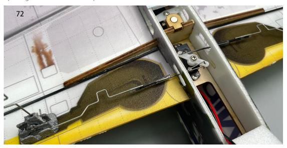
73. Adjust the length of both rods to ensure that the landing gear retracts and extends evenly into the correct position.
