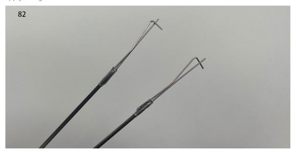
83. Install connection hooks on the tail control horns.
