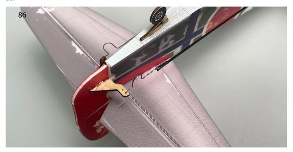
87. Install connection hooks on the aileron control horns.
