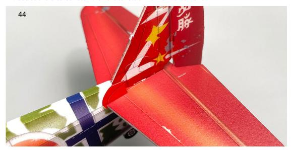
45. Use a sharp tool (screwdriver) to score along the wing's marked line, allowing the wing to fold downward along the center longitudinal line to form the airfoil.
