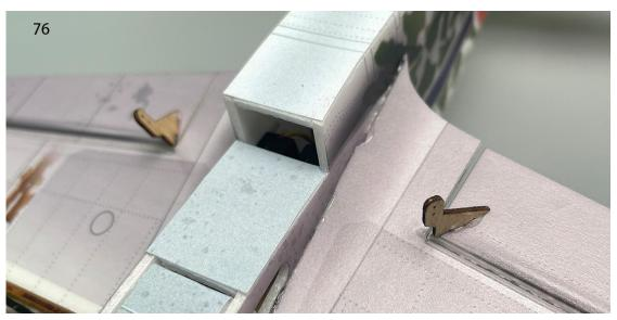
77. Install the horizontal stabilizer control horns.
