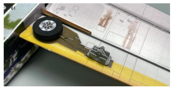
62. Check the operation of the landing gear servo while it is powered on to ensure it functions correctly (as shown in the diagram).
