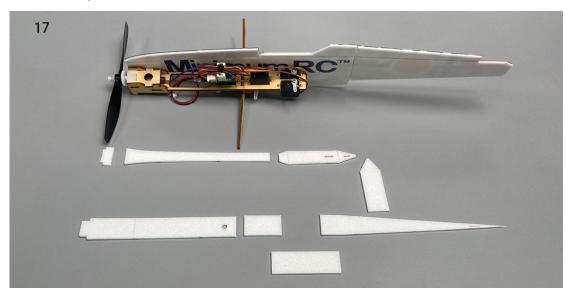
18. Press the fuselage inward along the score lines and use glue to install the bulkhead.
