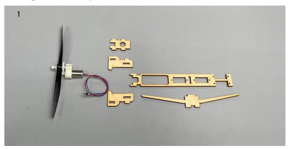
2. Assemble the fuselage wooden frame.
