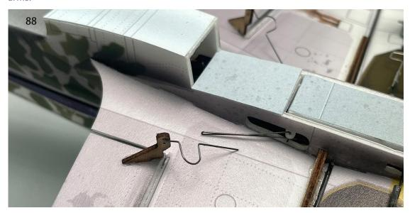
89. Use heat shrink tubing to connect the aileron wire clamp heads to the connection hooks, then apply 502 glue for fixation.
