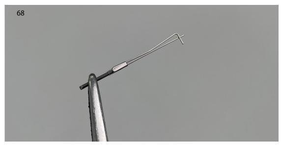
69. Install the rod end clamp onto the servo arm.
