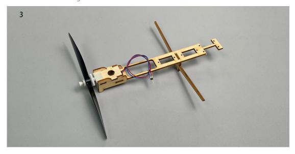
4. Install the servo as shown. (Top view of the parts)
