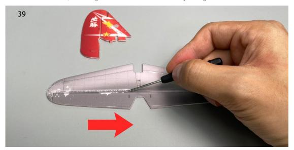
40. Use a sharp tool (screwdriver) to score through the marked lines on the bottom of the vertical stabilizer, allowing the rudder to move freely along the lines on both sides.
