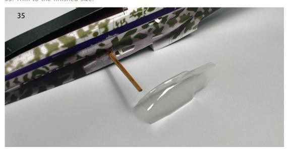
36. Install the canopy onto the fuselage at the corresponding location.
