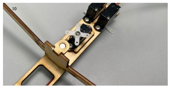
11. Connect the receiver to the servos, secure the receiver with Velcro, power it on, and bind it to the transmitter to ensure that the servo arms return to their neutral positions. Test if the servos are functioning correctly and install the servos and arms as shown in the diagram. Note: This step is crucial; make sure the servos are powered, the arms are centered, and follow the diagram precisely. Adjustments cannot be made after the model is assembled.
