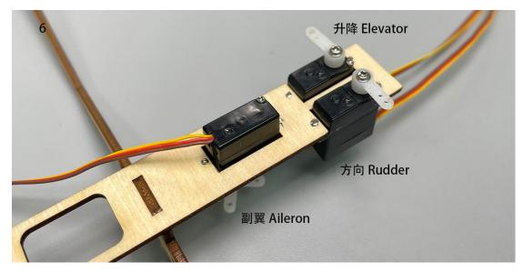
7. Install the servo as shown. (Bottom view of the parts)
