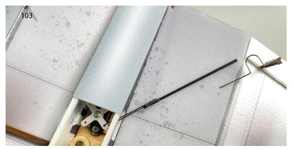
104.Use heat shrink tubing to connect the aileron wire clamp heads to the connection hooks, then apply 502 glue for fixation.
