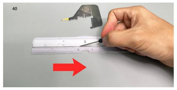
41. Use a sharp tool (screwdriver) to score through the marked lines on the bottom of the vertical stabilizer, allowing the rudder to move freely along the lines on both sides.
