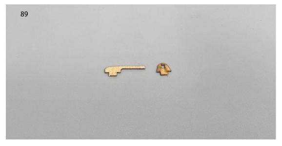
90. Install the aileron linkage parts.
