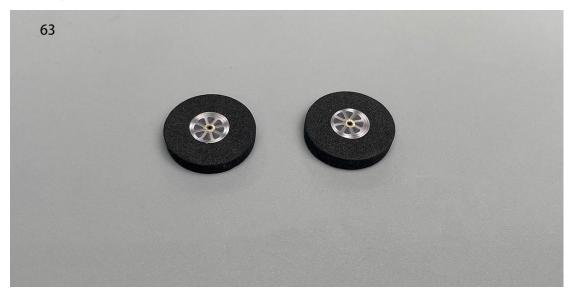
64. Install the wheels and bend the landing gear wire ends upward to prevent the wheels from coming off. Alternatively, cut a small piece of heat shrink tubing, slide it onto the end of the wire, shrink it, and apply a small amount of adhesive to prevent the wheels from coming off.
