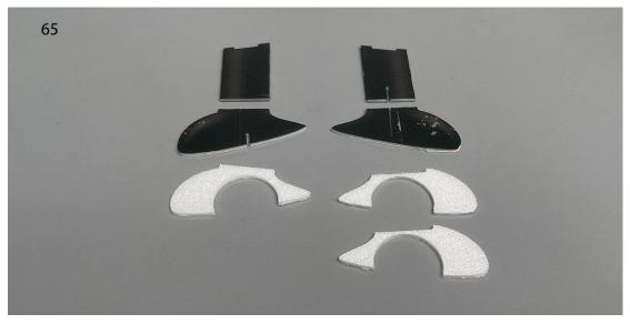
66. Overlap and bond two identical PS foam boards.
