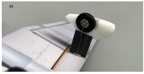
86. Install the thinner landing gear foam board component on the inner side of the landing gear.
