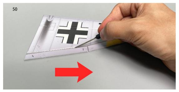
51. Use a sharp tool (screwdriver) to score along the aileron's marked line, allowing the aileron to move up and down along the line.
