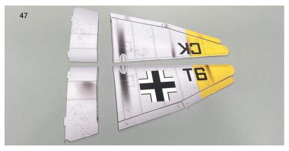
48.Use a sharp tool (screwdriver) to score along the wing's marked line, allowing the wing to fold downward along the center longitudinal line to form the airfoil.
