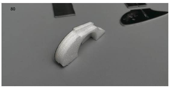
81. Use the engraved lines for assistance in positioning, install the landing gear support foam board, and pay attention to the front and rear orientation to avoid confusion.
