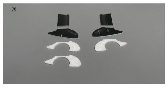
77. Overlap and bond two identical PS foam boards.
