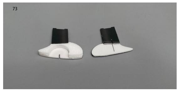
74. Install the thicker landing gear foam board component on the outer side of the landing gear.
