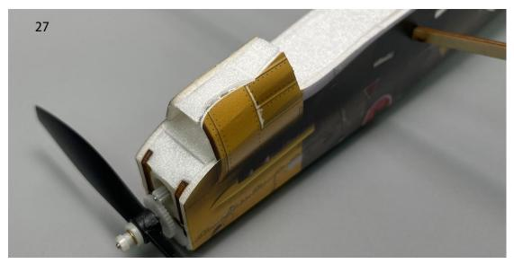
28. Remove the propeller and apply the fuselage stickers.
