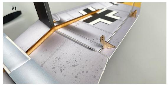
92. Install the rudder control horn.
