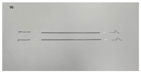
97. Use heat shrink tubing to connect the control rods and servo wire clamp heads, then apply 502 glue for fixation.
