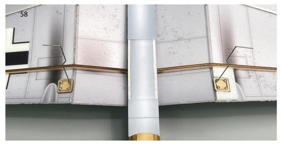
59. Adjust the landing gear wires to make them perpendicular to the ground.
