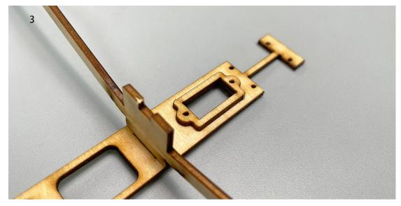
4. Continue assembling the wooden frame and install the motor.
