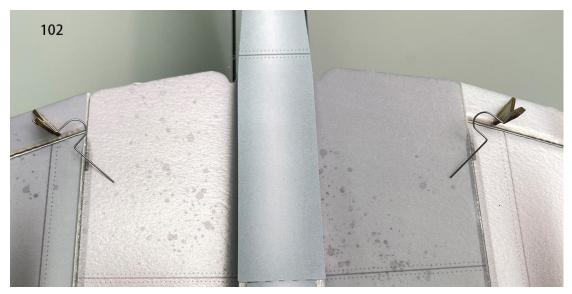
103. Insert the wire clamp heads into the fuselage and install them on the aileron servo arms.
