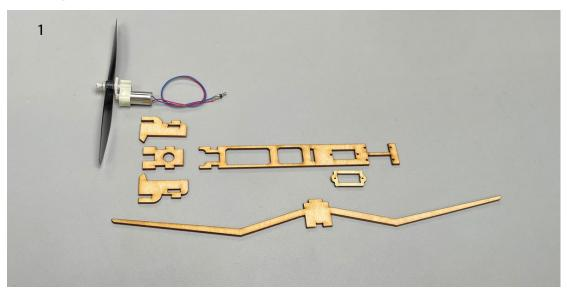
2. Assemble the fuselage wooden frame.
