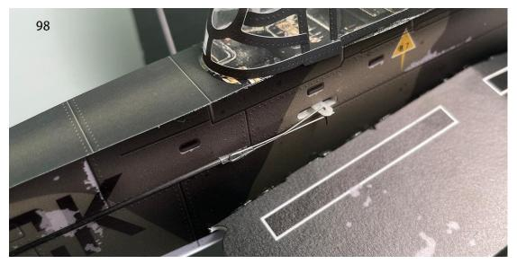
99. Trim the carbon fiber rod to the appropriate length. Use heat shrink tubing to connect the carbon fiber rod to the connection hook, then apply 502 glue for fixation.
