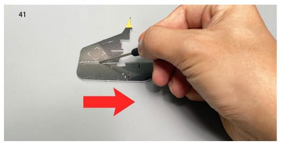
42.Install the vertical stabilizer reinforcement.
