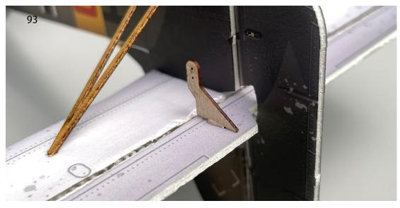
94. Install the rudder control horn connecting hook.
