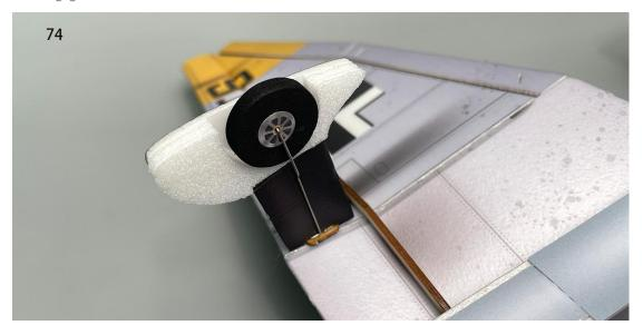
75. Install the thinner landing gear foam board component on the inner side of the landing gear.
