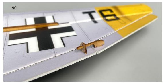
91. Install the aileron control horn.
