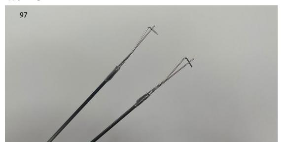
98.Mount the control rod clamp heads on the servo arms.
