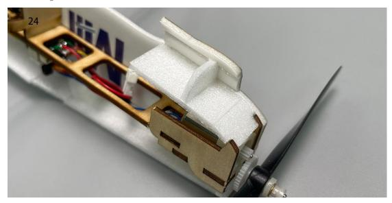
25.Use glue to secure the fuselage bottom plate, do not apply glue to the red-lined section.
