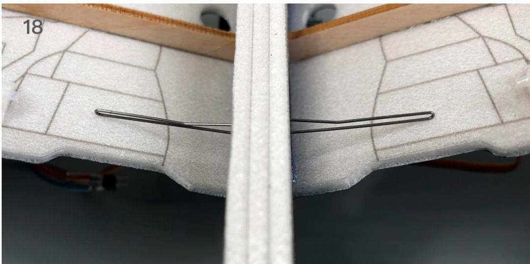
19. Attach the steel wire hooks to aileron control horns.
