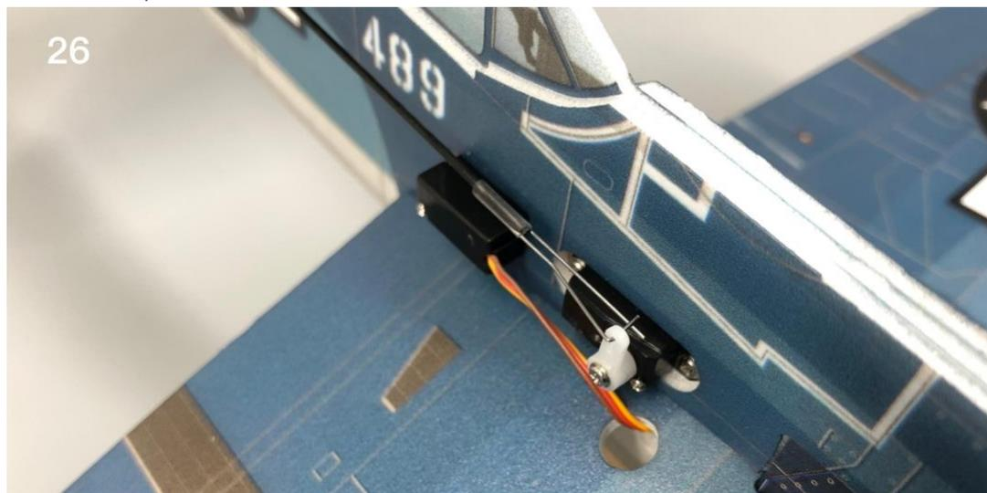
27. Attach the pushrods to control horns.
