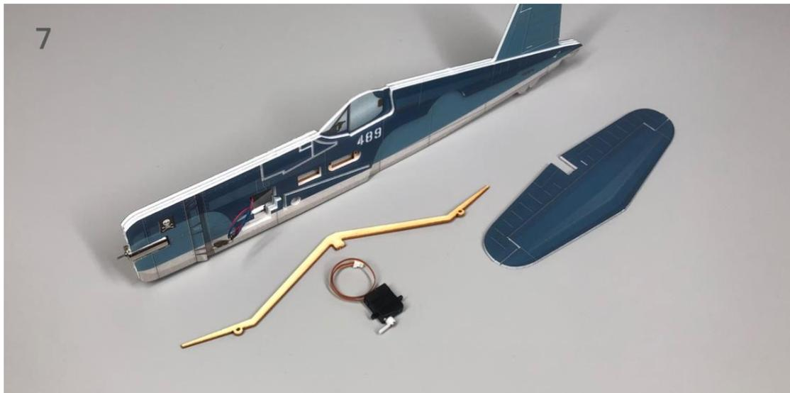
8. Install the aileron servo & wing support with glue.
