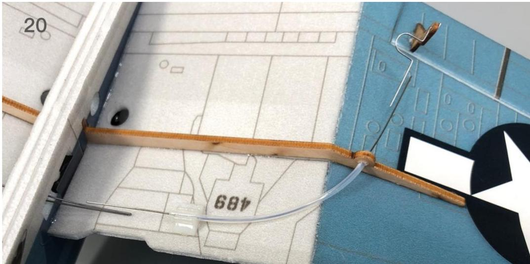
21. Connect the aileron servo to a powered receiver to make sure the servo arm is on its central position. Connect the steel wire and clips with heat-shrinkable tube and fix with glue. (Note: Using fire may damage foam material. Please use electric soldering iron.)
