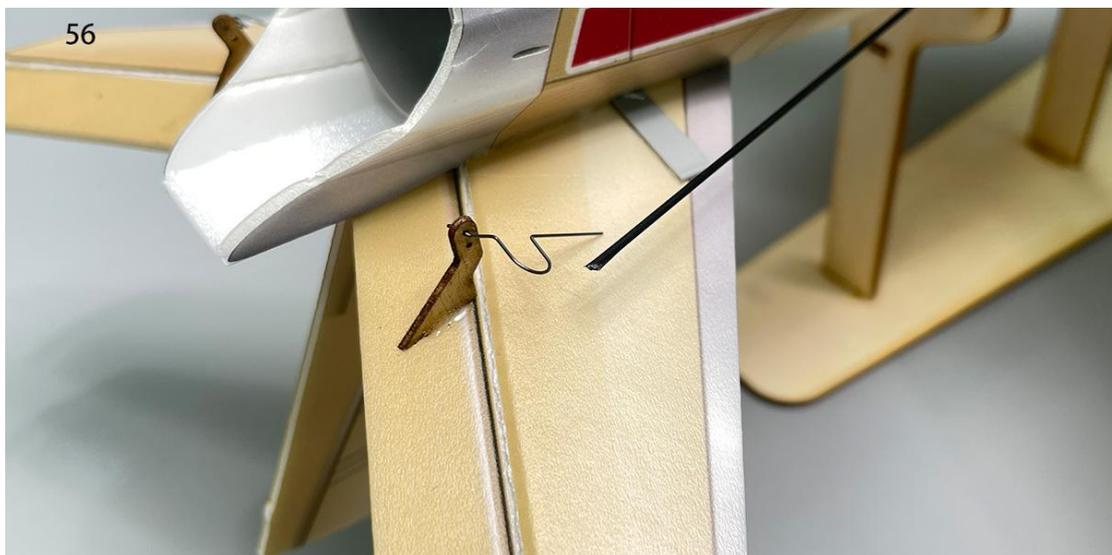
57. Use heat shrink tubing to connect the control rods to the connection hooks, then apply 502 glue for fixation.
