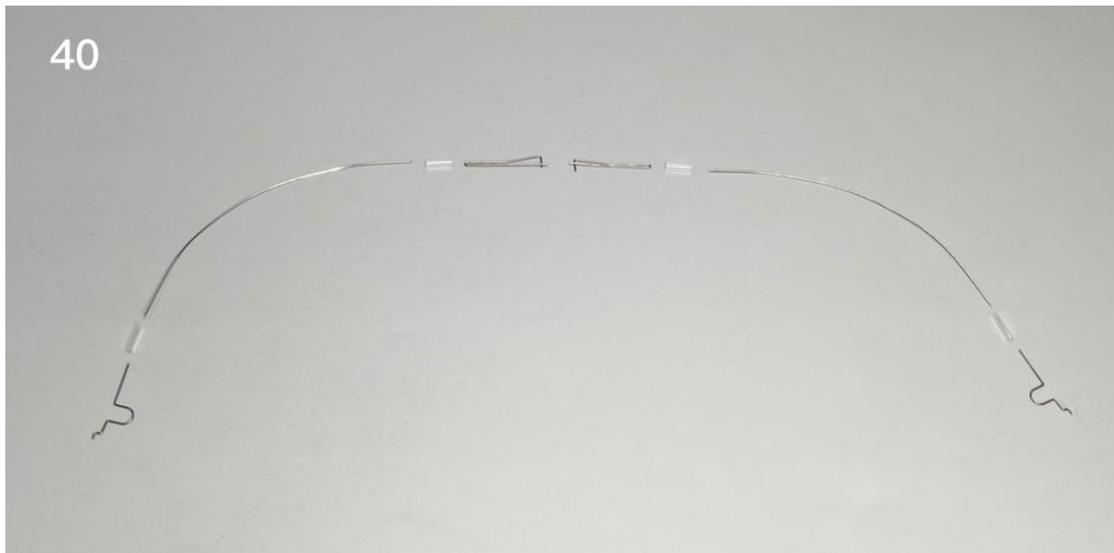
41. Connect the steel wire and a servo clip with heat-shrinkable tube and fix them with 502 glue.
