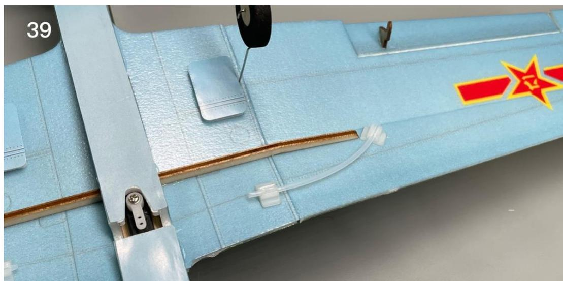
40. Aileron wire drive system. Bend the steel wire as shown to decrease resistance.
