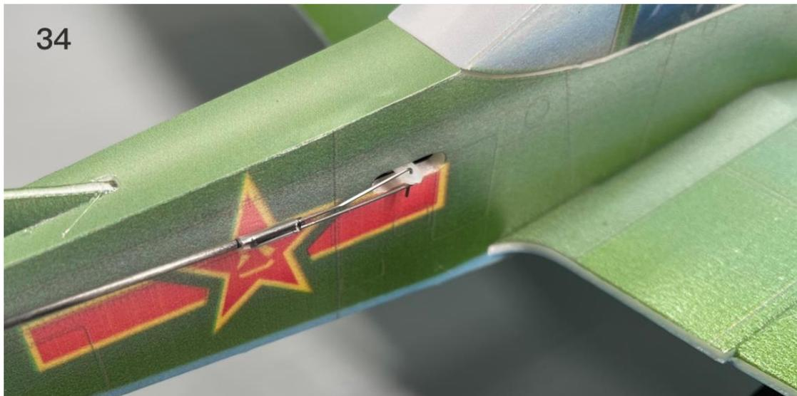
35. Connect the servo arm and control horn with pushrod.
