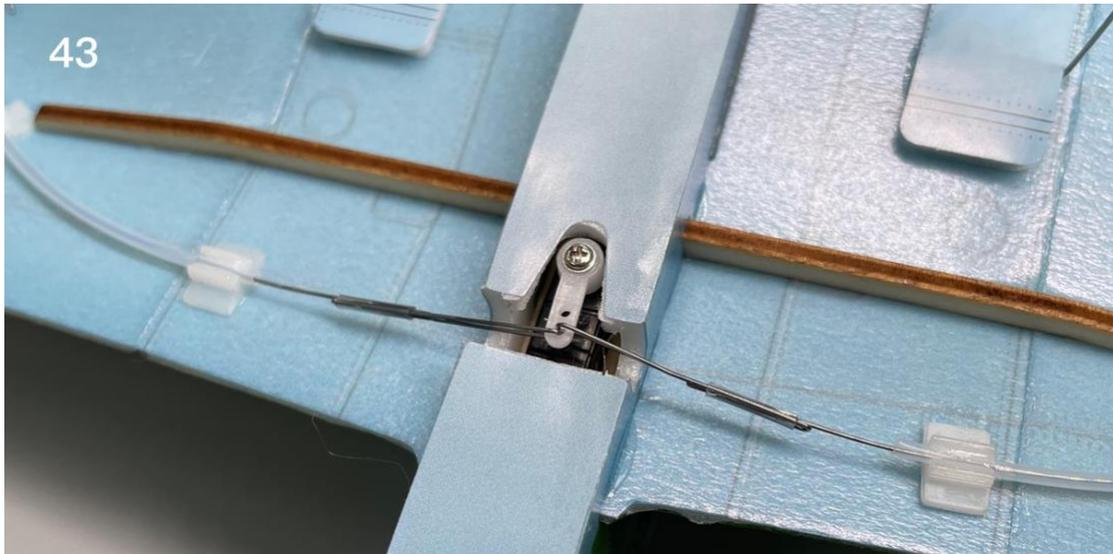
44. Connect the aileron servo to a powered receiver to make sure the servo arm is on its central position. Connect the steel wire and clips with heat-shrinkable tube and fix with glue. (Note: Using fire may damage foam material. Please use electric soldering iron.)
