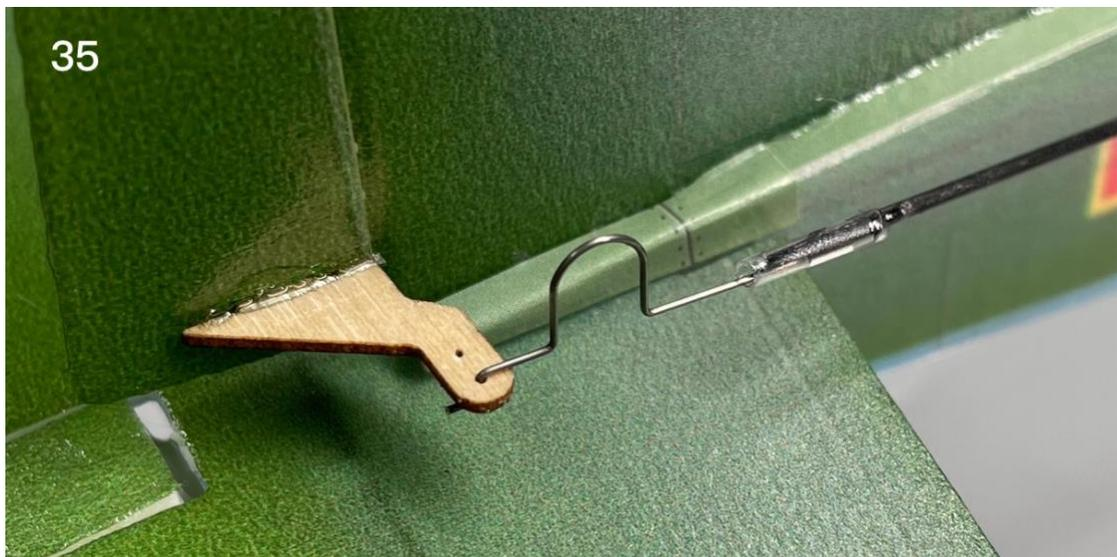
36. Install the aileron control horn.
