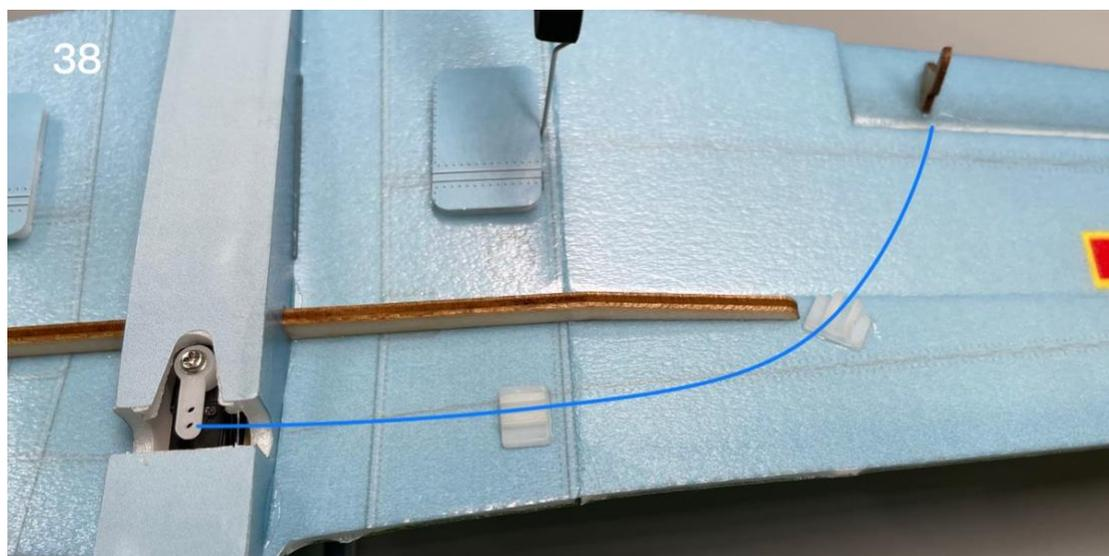
39. Use 502 glue to fix the conduit on the base. Note that 502 glue is not accessible to foam parts.
