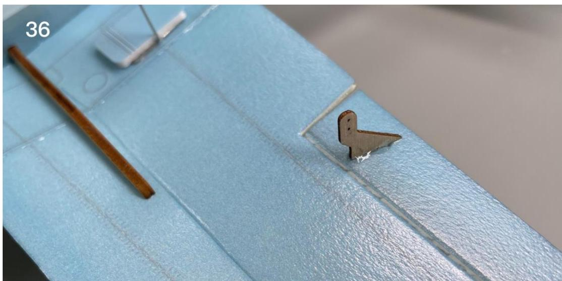
37. Use UFO glue to fix the conduit base according to the position shown.
