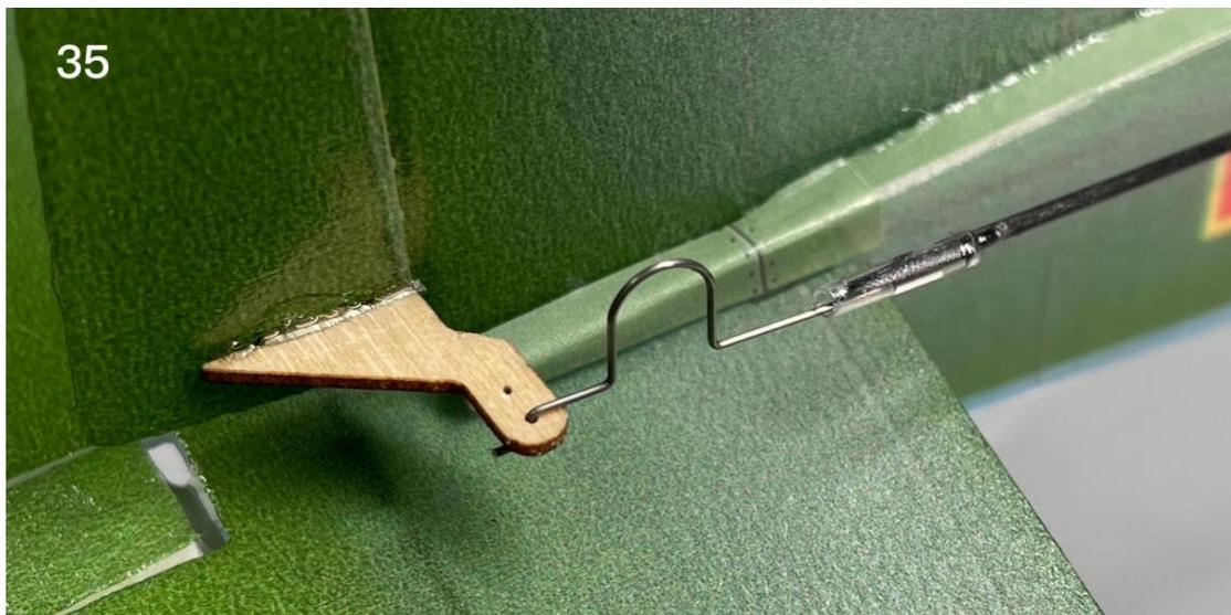
36. Install the aileron control horn.
