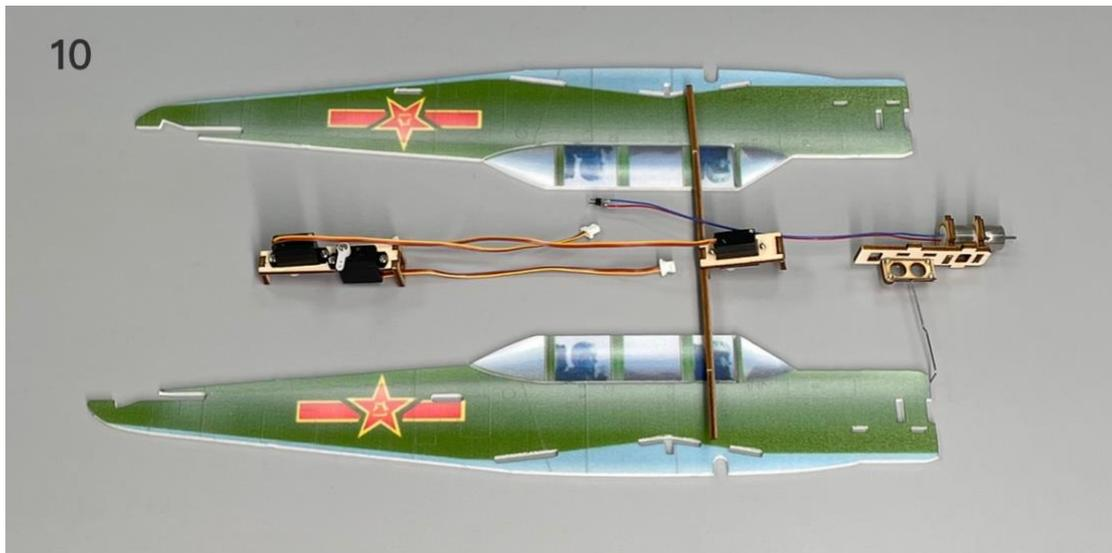
11. Install the fuselage internals according to the marked position inside the fuselage
