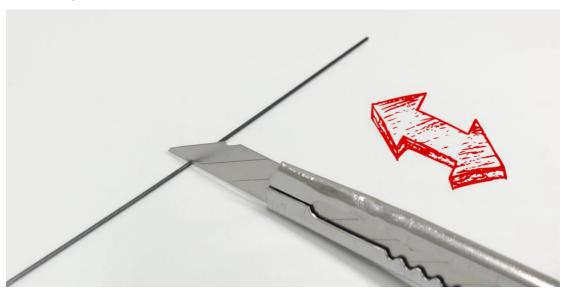
3. Divide φ0.8mm carbon rod into: 2x 425mm; 2x 300mm; 1x 117mm; 1x 38mm; 1x 31mm.
