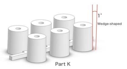
24. The propeller adapter is wedge-shaped and is installed with the smaller end facing forward.
