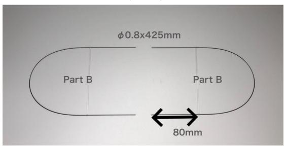
18. Use heat-shrink tube to connect the wings on both sides and glue with 502 glue.
