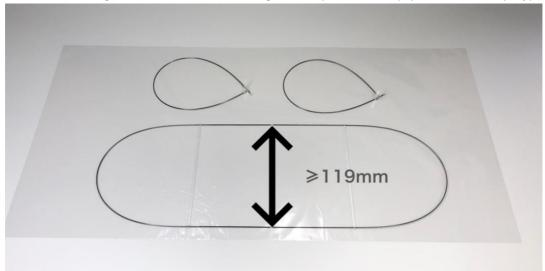
33. The excess film is cut along the outside of the profile to obtain a complete wing & tail. When the wing is installed, the film side is facing up.
