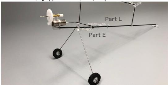
12. Take two  $\phi$ 0.8x300mm carbon rods, combine with part C, and fix with 502 glue.
