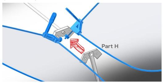
16. Use the screws to secure part H to form a full-motion V-tail.
