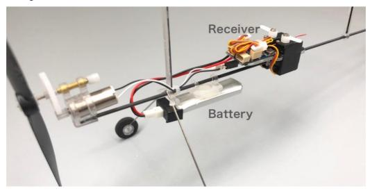
27. Use heat-shrinkable tube to connect the  $\phi1mm$  carbon rod to the clips. Note: The length of the push rods needs to be cut according to the actual demand.
