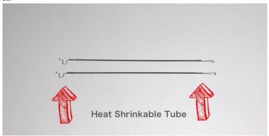
29. Connect the push rods to the tail. It is recommended to use the connection hole at the top of the rudder arm.
