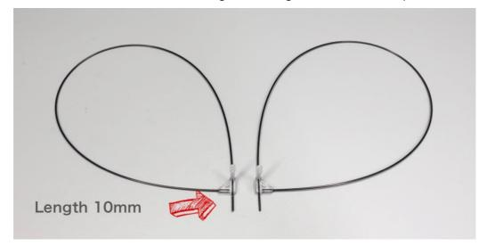
14. The carbon rod end stopper (part G) has a gap of 4-5 mm between the stopper and the bracket. (Please read step 13 before bonding)
