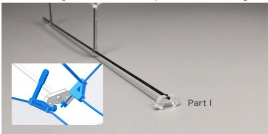
8. Assemble the landing gear. Use heat-shrinkable tube to hold the wheels.
