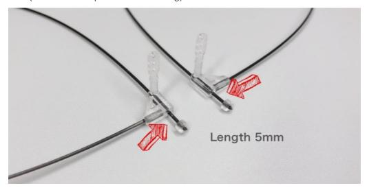
15. The root of the tail fin needs to be inserted into the groove of part I, and it can rotate freely without sticking. Excess carbon rods are removed at the end.
