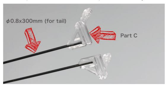
13. Bend the carbon into tail frame; The end of the carbon rod is extended by 10 mm. Note: The direction of carbon rod bending is confusing. Please observe the picture.
