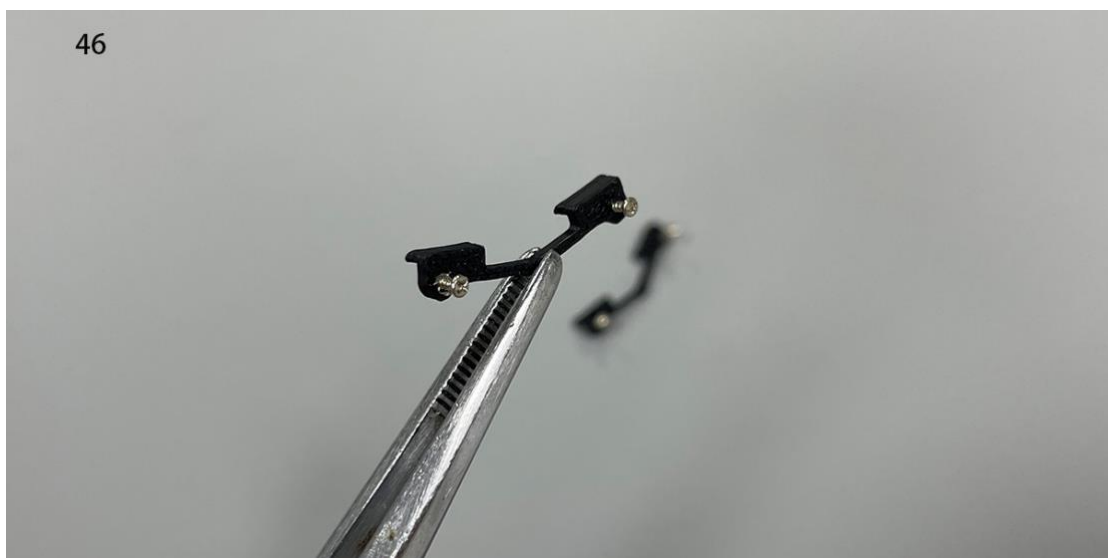
46. Install two m1x3 screws on the wing fixing piece L.
