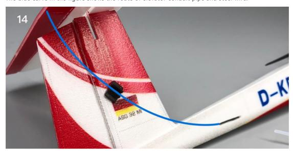
15. Glue the conduit to the conduit base inside the fuselage, and the two ends of the conduit pass through the two conduit holes on the right side of the fuselage.
