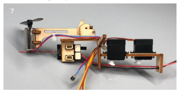
8.Connect the cable of servos and motor, and connect the receiver to power for test. Ensure that the servos and motor work normally and the motor rotation direction is correct.
