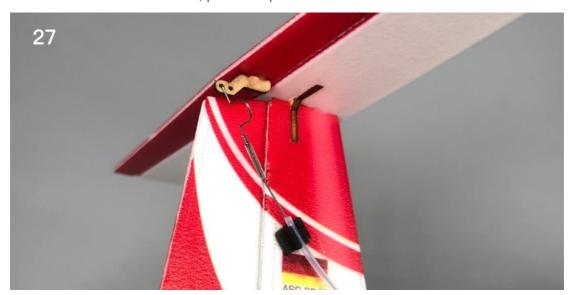
28. Connect the pushrod clip, steel wire and servo arm.
