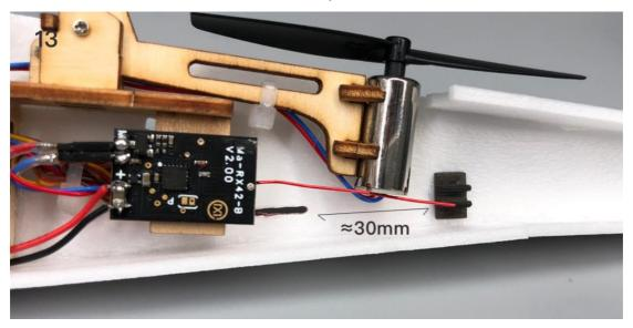
14. As shown in the figure, paste a duct seat on the right side of the vertical tail. This guide socket is used to fix the end of elevator drive pipe.
