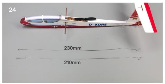
25. Thread the steel wire into the conduit on the fuselage. The steel wire is used for elevator drive, and the shorter one is used for rudder drive.
