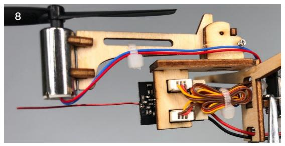
9. Combine the fuselage inner structure with the right panel of the fuselage.Note: the bottom of inner structure (red circles) should be 2mm away from the edge.
