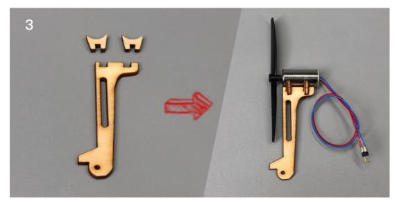
4. Use m1.2x6mm screw to fix the turnover motor base. Adjust the distance between the fixed pieces on both sides of the motor base till the motor base can be turned over freely. If necessary, sand the motor base to reduce its thickness to make the turning movement smooth.
