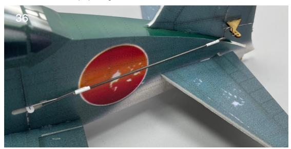
37. Use heat shrinkable tube to connect aileron steel wire clips.
