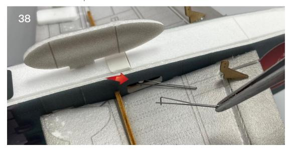
39. Connect the wire hooks with heat shrinkable tubes.
