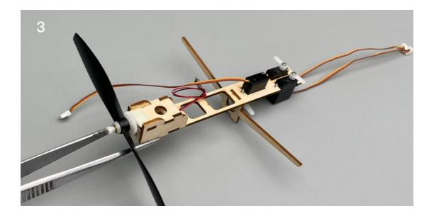
4. (bottom view) the three servos are installed and fixed under the plywood board.
