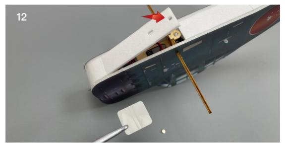
13. The battery cover can be opened, and can be adsorbed in the closed position by magnet.
