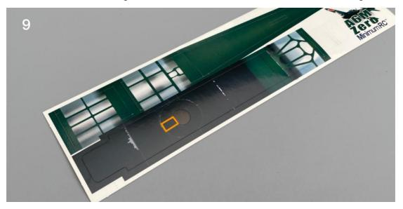
9. Cut out the illustrated orange area on the sticker to avoid interference with the motor gears.
