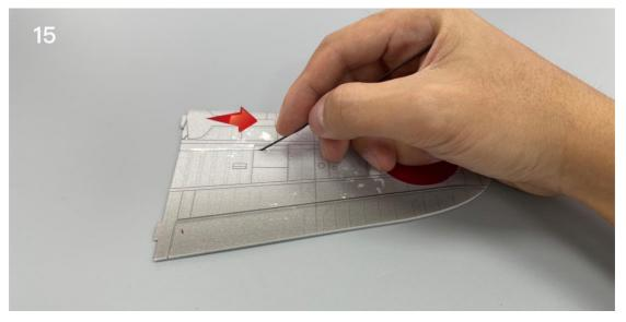
16.Use the end of a carbon fiber rod to score through the aileron half-cut line of the wing surface.
