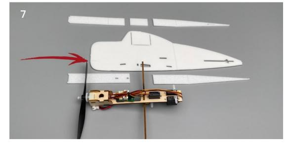
7. Align the scribed line on the inner side of the fuselage and fix the wooden structure with glue.
